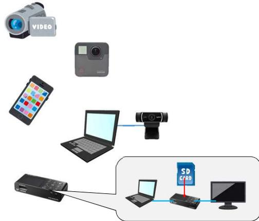
The diagram illustrates the equipment needed for video capture. It includes a video camera, a live camera, a smartphone, a laptop with a capture card, and a dedicated video capture device connected to a laptop and monitor. A callout box shows the capture device connected to a laptop and monitor, with an SD card icon indicating data transfer.
